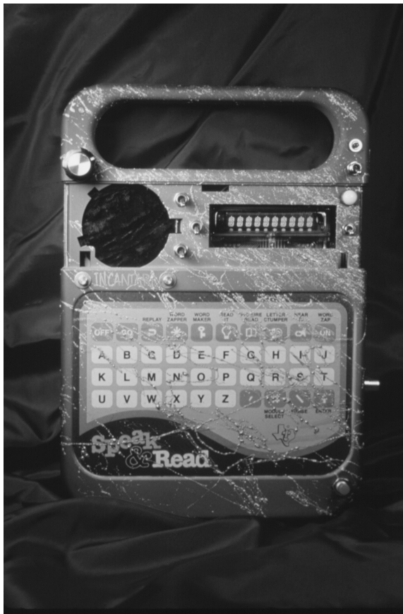
Fig. 7. Modern Incantor, circuit-bent Speak & Read, electric eye in antique brass and milk glass lens, switches, potentiometer, LEDs, paints, holographic dusts, approx. 7 \times 10.5 \times 2 in, ca. late 1980s. (© Qubais Reed Ghazala) The looping system consists of the four controls to the upper right; the streaming switches are centrally located; the pitch dial and body contacts are further to the left. Its reset button, a simple power-supply interrupter, is to the lower right.
