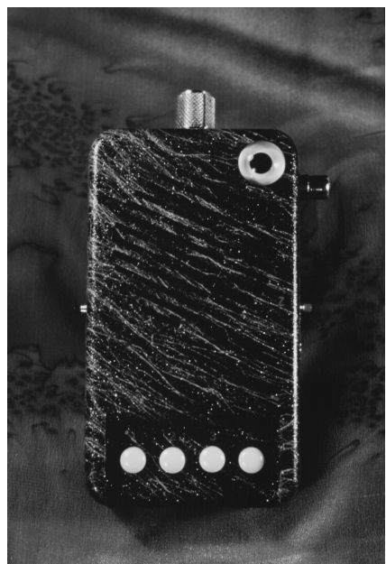
Fig. 4. Inverter, circuit-bent toy containing audio samples of human voice and automotive sounds with push-button switches, glass fish eye, potentiometer, paints, approx. 3 × 5.5 × 1.5 in, ca. early 1990s. (© Qubais Reed Ghazala) The Inverter is a “living instrument” whose new wiring creates thermal pressures upon the circuit, changing its voice over time.
