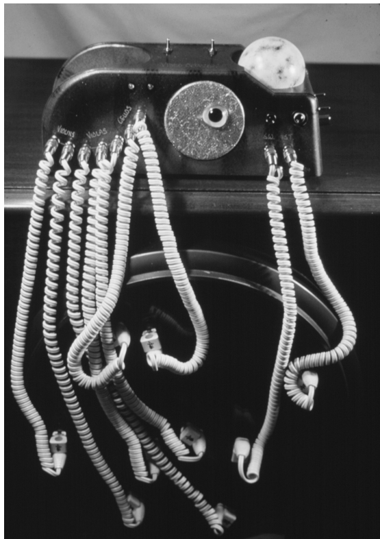
Fig. 12. Video Octavox, antique telephone amplifier case, glass fish eye, coil cords with photo-sensors, painted wooden model of the sun, miniature footlights for the sun, antique faceted glass lenses, LEDs, nine potentiometers, eight antique brown Bakelite knobs (on back), eight line outputs (on back), original circuit, approx. 9 × 5 × 4 in, ca. late 1980s. (© Qubais Reed Ghazala) This instrument is designed to use a videotape or a DVD as a score; it can also use random events (e.g. via video camera) to produce an aleatoric "string ensemble" response.
