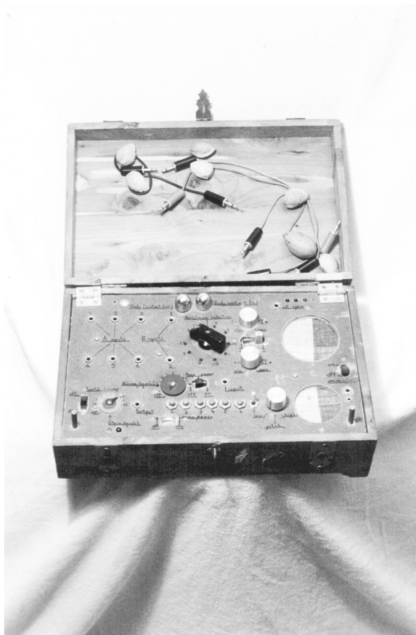
Fig. 2. Original circuit now re-fitted into permanent housing, circuit-bent transistorized 9V amplifier, cedar box, orange plaid curtain material, almonds and pecans in the shell, 1/8-in patch cords, chrome hemispheres for body contacts, various switches and potentiometers, two 3-in speakers, approx. 11 × 5 (closed) × 8 in, ca. 1968. (© Qubais Reed Ghazala) Armored now against attacks, the instrument settled into this final configuration, surviving to the present day.
